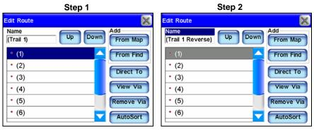
1. Select the NAME box and use the virtual keyboard to change the route name from "(Trail 1)" to "(Trail 1 Reverse)". Changing the name helps you tell a forward route from a reversed route. The parentheses () indicate this route was made from a trail. 2. Select point 1 and press the DOWN button to move it to the bottom of the list.
